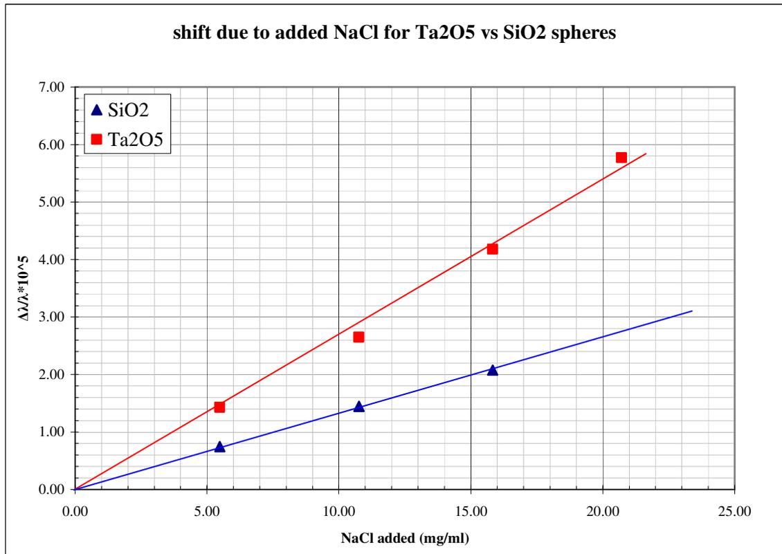
Figure 3.8 fractional resonance shift due to NaCl addition
